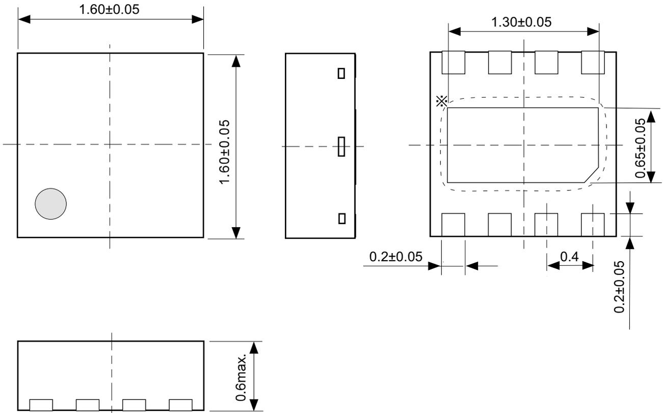
※ The heat sink of back side has different electric potential depending on the product.
