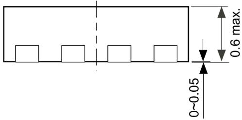
※ The heat sink of back side has different electric potential depending on the product. Confirm specifications of each product. Do not use it as the function of electrode.
